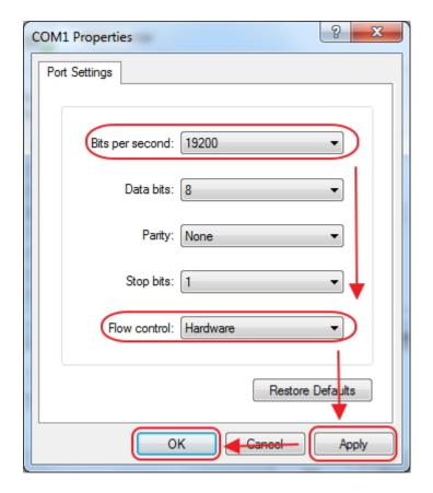
"Bit per second" means Serial port baud rate, it must same as printer setting. For example, if printer baud rate is "19200bsp", then you must select "19200" on "Bit per second", just as above picture. (Factory default baud rate is 19200bps)
