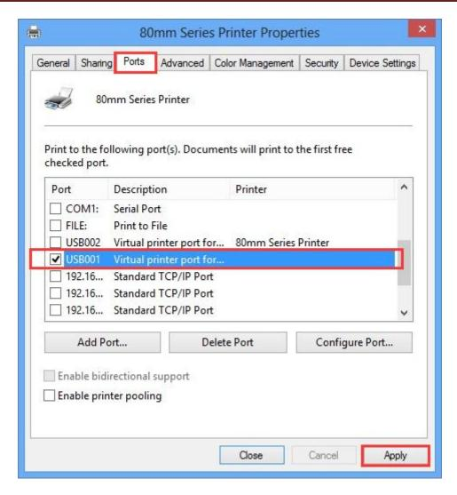
Select available computer USB communication port, such as the above picture shows "USB001", and then click "Apply" to finish the configuration.
