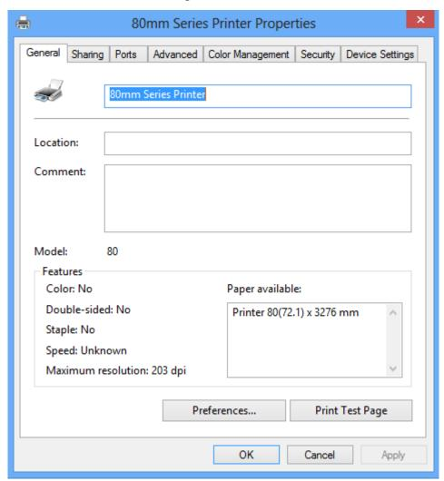
On 80mm Series Printer Properties "General", you could configure the printer communication port, such as Serial port, Parallel port and USB port. You also could set the paper specification, beeper etc.
