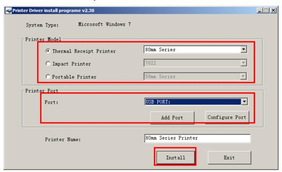
Select the Printer Model and available printer port, such as "USB PORT" as the below picture, Then, click "Install".
