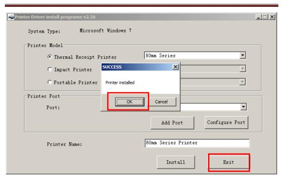
Select "OK", and then click "Exit". Wait till it shows the below picture, it means, the printer driver has been installed successfully.
